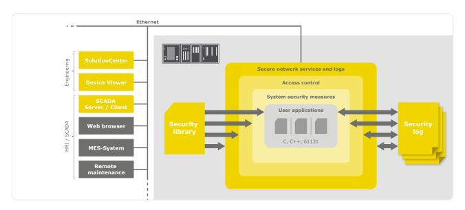
The layer-based security architecture forms multiple security walls around user applications. Each level includes specific security measures that can also be used in user-specific applications.
