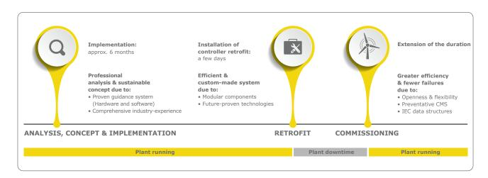
With appropriate preparation the actual upgrade of the turbine with a new controller system requires only a few days on which the turbine is off grid.
