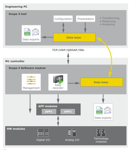
The central aspect of Scope 3 is the portable database on the Engineering PC and M1 controller. This enables very simple data exchange and collaboration – also using copies of a single file, if necessary.
