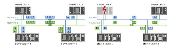
✓ Switchover of the active CPU within a PLC cycle, e.g. cycle time 1 ms – switchover ≤1 ms
