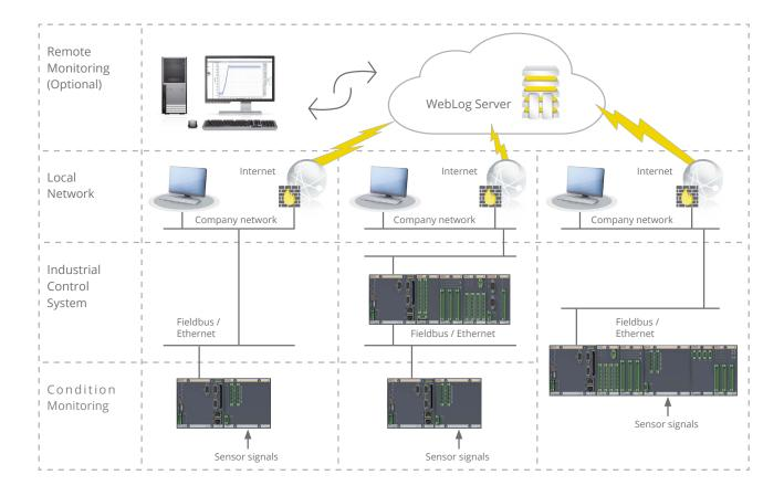
The AIC214 system concept allows a free design of the condition monitoring software to the requirements of a specific application.
