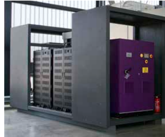
Test rig for lithium ion batteries in the Younicos Technology Center in Berlin-Adlershof.
