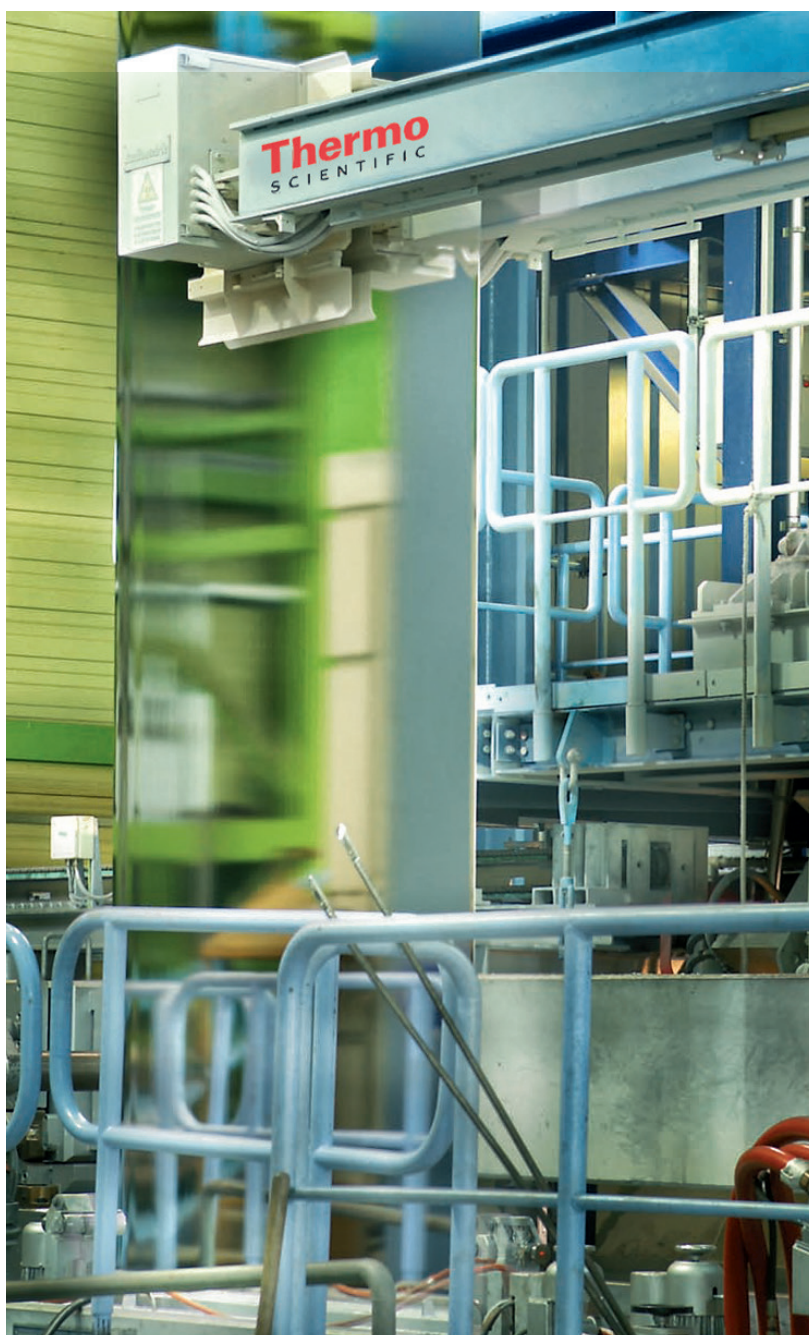
▲ Thermo Scientific Sipro gauges for hot strip lines. The upper arm in the photo contains the two X-ray sources. The detector arrays are located in the other arm below the hot strip. The gauging system delivers the hot strip thickness cross profiles every 5 milliseconds.
