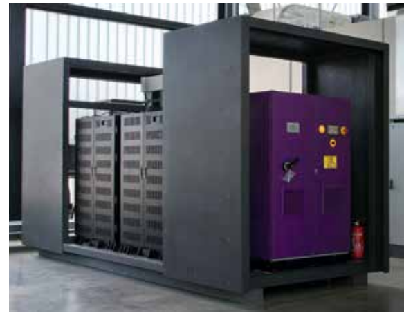
▲ Test rig for lithium-ion batteries in the Younicos Technology Center in Berlin-Adlershof.
