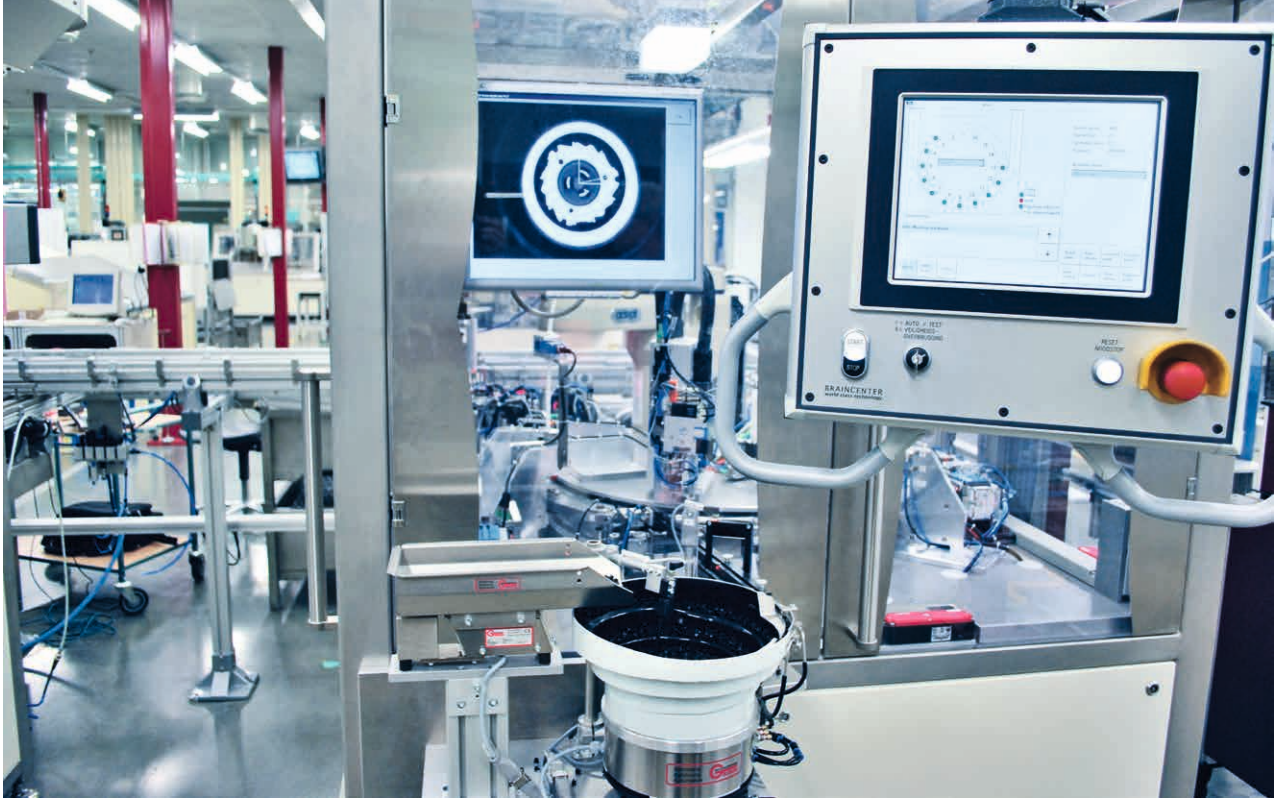
▲ Controlled with cameras: Production quality and parts orientation are monitored during shaver head assembly.
