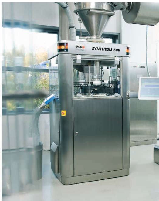
▲ Synthesis 500 ZSM: Two-layer encapsulated core tablet press from Kilian with the safety controller system from Bachmann.
