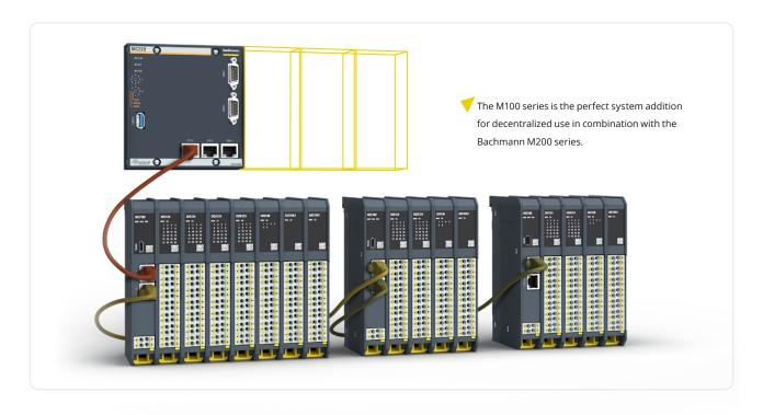
The NEC102 node adapter maps the powerful and flexibly configurable M100 station to a standard EtherCAT interface. The operating modes of the M100 I/O modules are defined during the configuration and are available to both the Bachmann master and also to masters of other manufacturers. Thanks to distributed clocks on the EtherCAT stations that can also be synchronized with external time servers, the implementation of short control intervals across the entire control system is given.
