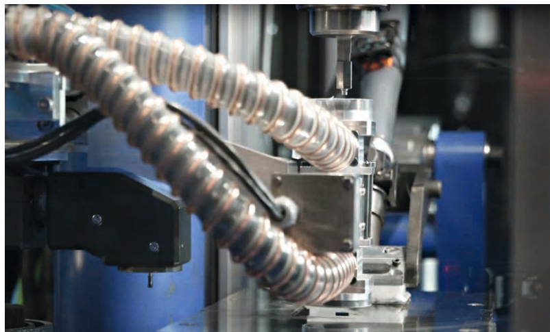
The integrated brushes clean any shape, no matter how complex, close to the contour, removing a powder residue from the pressing area.
