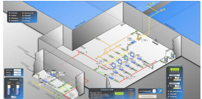
Everything in view: Approximately 100 station visuals are displayed three-dimensionally and approximately to scale with atvise®.
