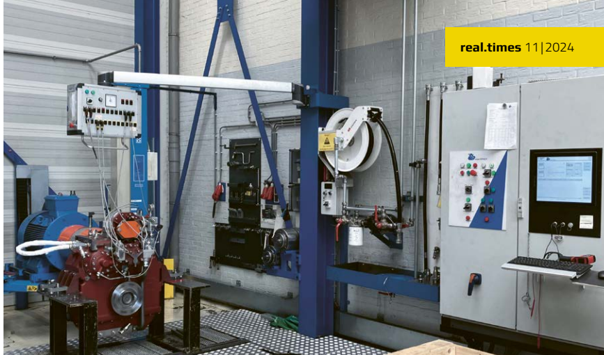
Gearbox test bench implemented by Verhoef Elektrotechniek: Whereas testing used to be documented manually by the operating personnel, customers now automatically receive a detailed PDF report of the complete test, including clutch engagement and disengagement trends thanks to WebMI pro and Scope 3. © ADS van STIGT
