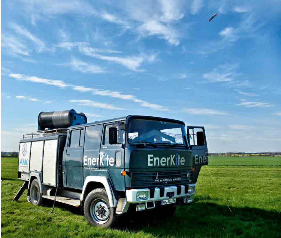
▲ For the test run EnerKite uses a truck as the ground unit where the electricity is produced by a generator.
