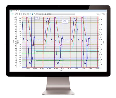
▶ High precision: The time relationships of various process variables are analyzed and the exact values can be read out with the measuring cursor.
