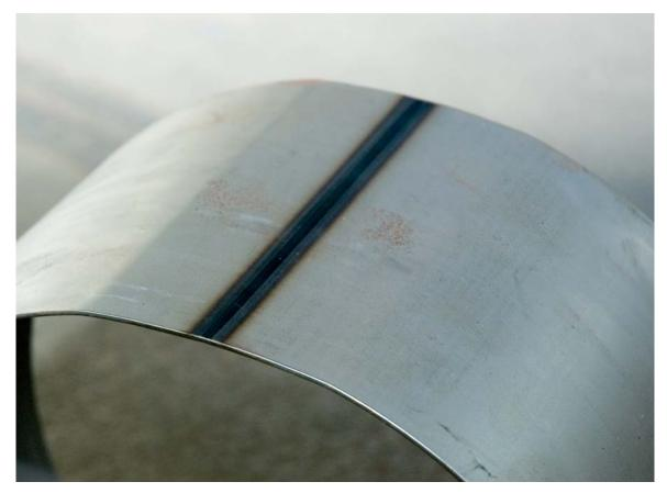
Welded cylindrical steel rim blank
