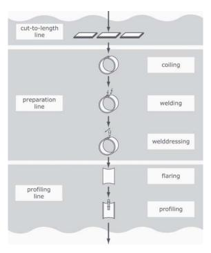
Detail of the production process of a steel rim: welding is the central process
