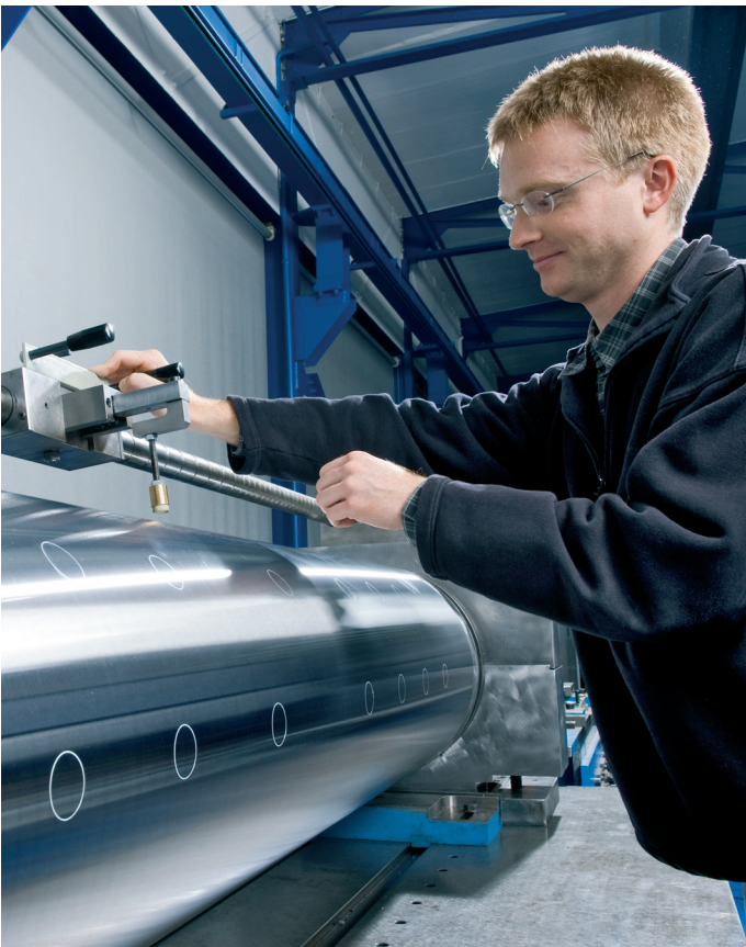
▲ Ingenious lay-out of sensors: Achenbach technician Tim Schuhmacher calibrates an evenness measuring roll
