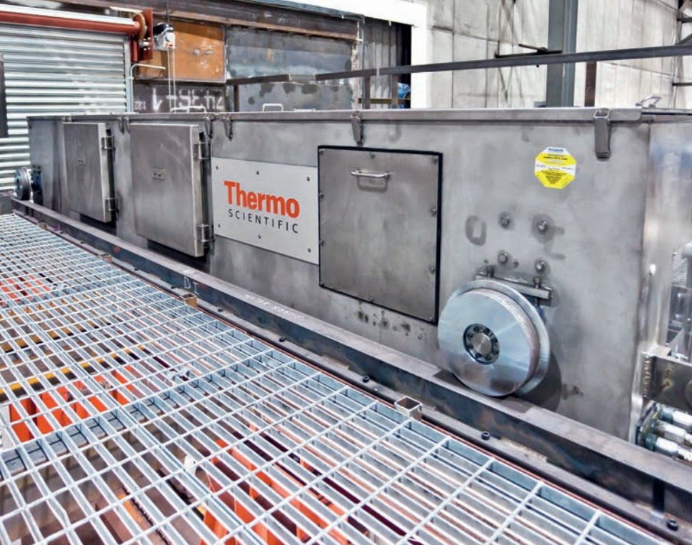
◀ Thermo Scientific SIPRO gauges for hot strip lines. The upper arm in the photo contains the two X-ray sources. The detector arrays are located in the other arm below the hot strip. The gauge system delivers the hot strip thickness cross profiles every 5 milliseconds.
