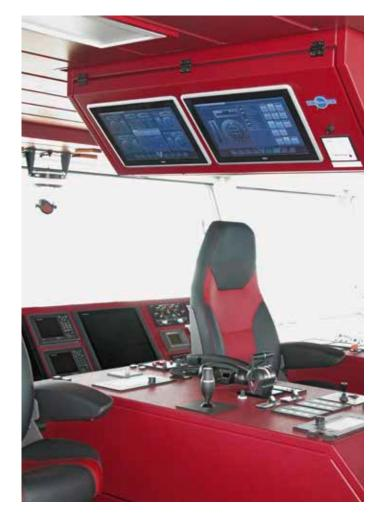
■ The M1 automation system is installed in the engine room where it records all the operating data and any faults. The monitoring can be carried out from the bridge as well as in the engine or propeller room. M1 webMI pro also enables remote access for service and maintenance at any time.
