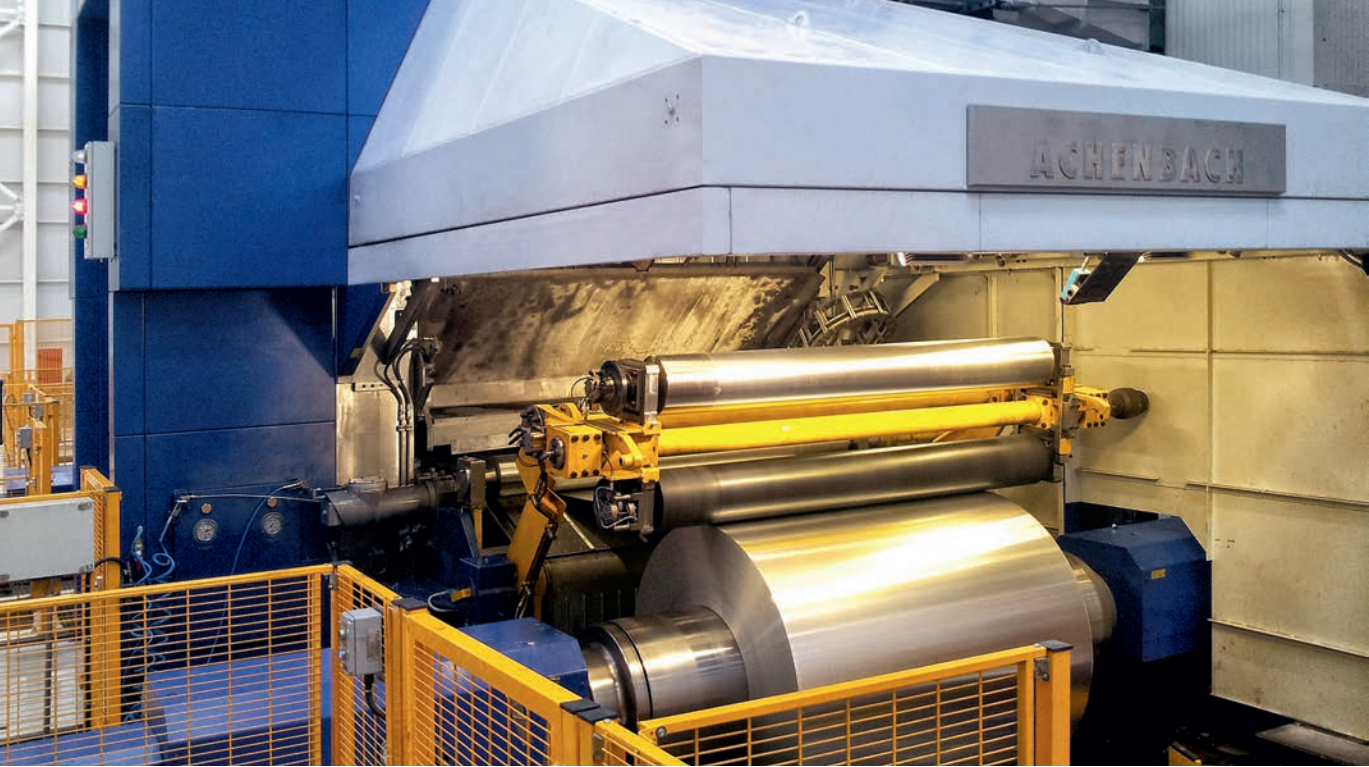
▲ Aluminum foil rolling mill: State-of-the-art measuring technology and the powerful M1 controller system used in innovative machinery enable maximum plant productivity and rolled products of the highest quality.
