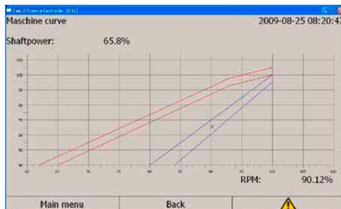
▲ Clear graphics indicate deviations from the ideal operating point and thus enable the optimization of fuel consumption: Display of the shaft power as a function of engine speed. Operating limits and the overload curve are included as a reference.
