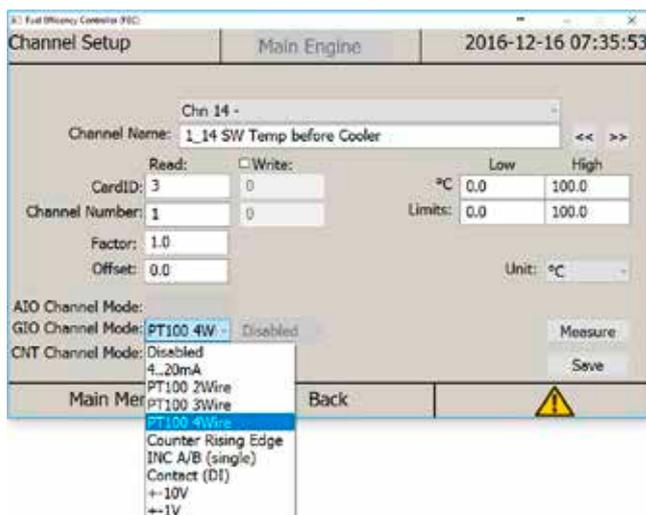
▲ The software modules can be assigned parameters as required via PC or touch screen without having to change the code on the PLC. This is critical since incorrect signal specifications can be adjusted by the ship's crew during a retrofit.
