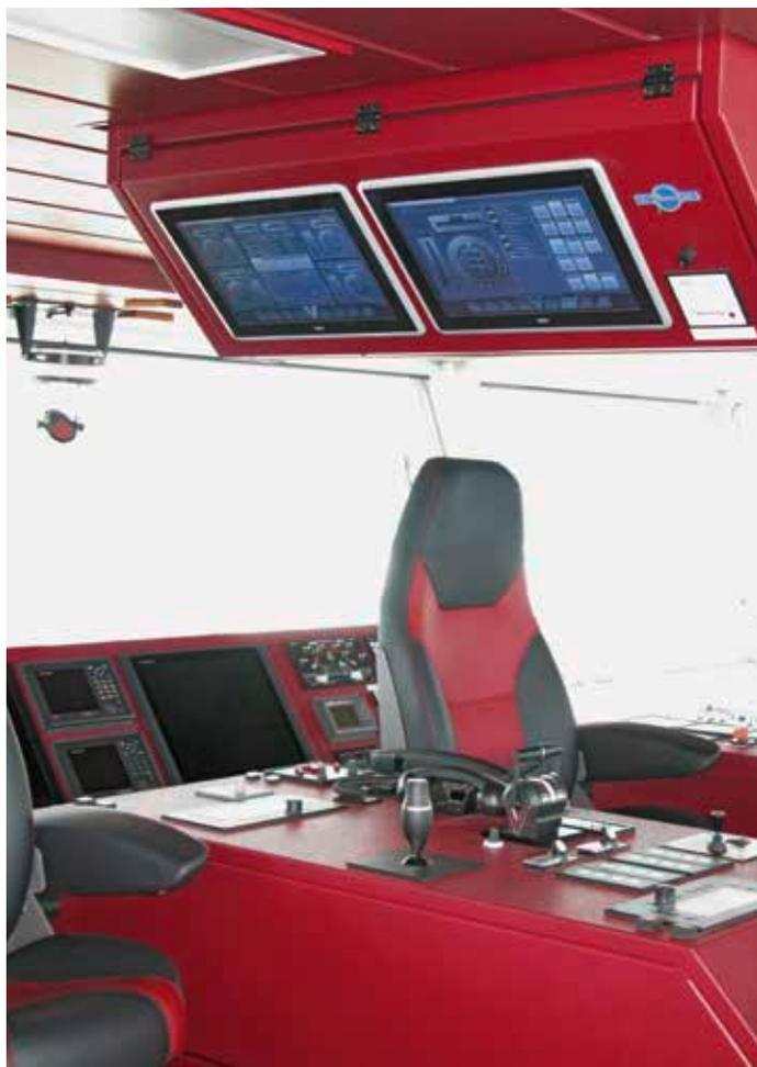
◀ The M1 automation system is installed in the engine room where it records all the operating data and any faults. The monitoring can be carried out from the bridge as well as in the engine or propeller room. M1 webMI pro also enables remote access for service and maintenance at any time.
