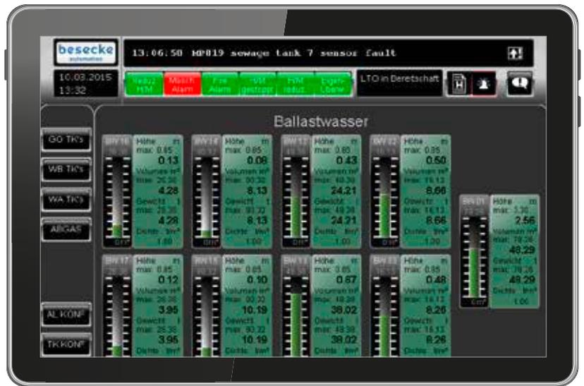
▲ The new operator interface is clearly designed and meets the requirements of the skipper. Alarms in the event of faults or limit value violations are recognizable at a glance.
