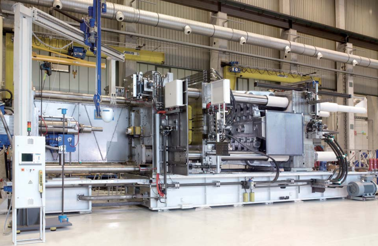
◀ GDK cold chamber die-casting machine from Frech: Up to 5,000 tons (50,000 kN) closing force. (construction in the assembly plant prior to painting.)
