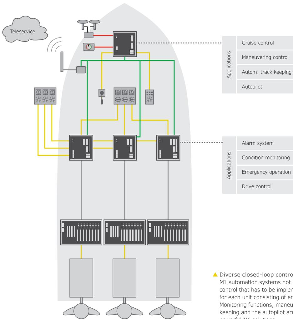
▲ Diverse closed-loop control tasks on a ship: M1 automation systems not only handle the drive control that has to be implemented separately for each unit consisting of engine and propeller. Monitoring functions, maneuvering control, track keeping and the autopilot are also controlled by powerful M1 solutions.
