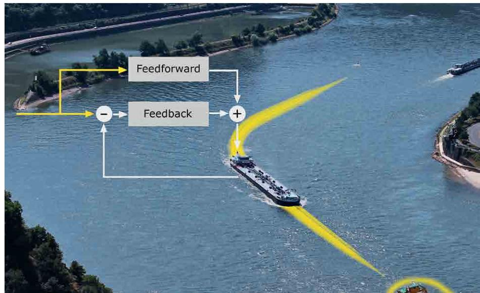
► Precision: Using the results of the position calculation, the track keeping system is able to detect deviations from the ideal course. From this the control algorithm forms manipulated variables for the rudder and keeps the ship on track.
