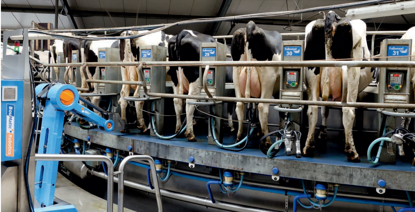
▲ The SR-1 spray robot precisely cleans the udder of the cow straight after milking and prevents the growth of infections. The robot is integrated in the rotary milking system, but functions completely independently.
