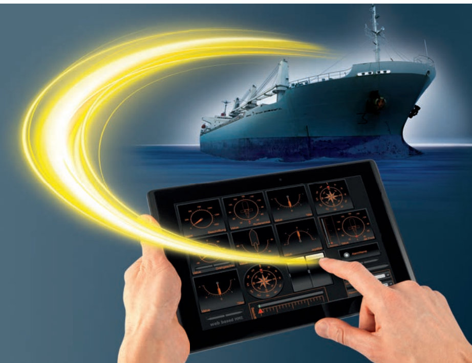
▼ State-of-the-art visualization solution on an Apple iPad™: HMI for propulsion controls on ships.
